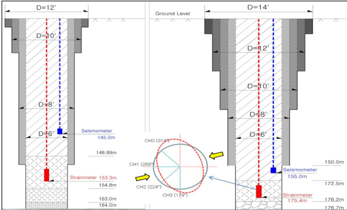
**Fig. 14.** Cross-sectional diagram of the borehole seismometer (blue) and strainmeter (red) installed at EF01 (left) and EF02 (right).
