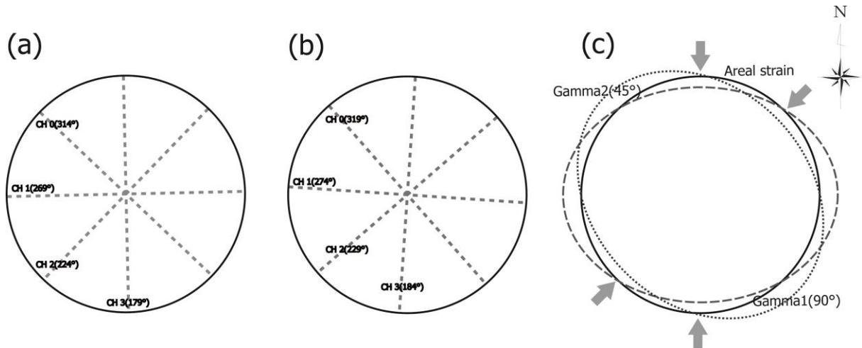
**Fig. 15.** Schematic map of strainmeter sensor direction. (a) EF01 station, (b) EF02 station and (c) converted strain field direction
