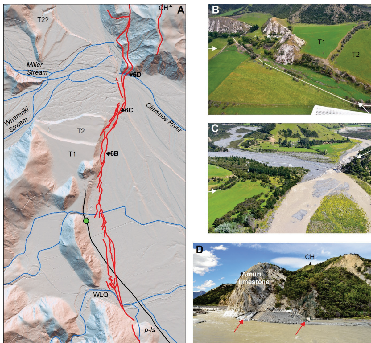
Figure 4.1 The Papatea Fault in the Middle Hill area. A. Rupture map from the Waipapa Quarry (WLQ) area to the Clarence River crossing near Corner Hill (CH) presented on a post-earthquake LiDAR hillshade model. Green dot is Stop 5 at Middle Hill Station (MHS). Asterisks mark the photo centres for B, C and D. T1 and T2 are two terraces elevated on the hangingwall side of the Papatea Fault. Abbreviation: p-ls, paleo-landslide deposit. B. Reverse and thrust fault rupture traces in front of MHS. C. Rupture traces progressing from MHS to the Clarence River; note the highly uplifted beds of the co-joined Miller and Wharekiri streams. D. Papatea Fault exposure on the NE bank of the Clarence River. Note the pair of rupture planes, and the uplift markers both within the fault zone and upstream where Amuri limestone bedrock has been uplifted. The red arrows mark two distinct fault zones (or the width of the entire fault zone).
