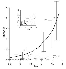
Fig. 2: Surface throw as a function of moment magnitude. Lines represent the model prediction, the symbols represent the data. For convenience, an enlargement is shown in the inset.
