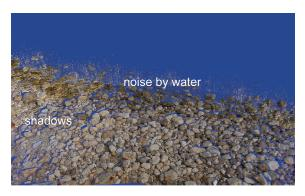
Fig. 5: Two major methodological problems arose in coastal monitoring using TLS in littoral zones: noise caused by water and shadowing effects by coarse material in the upper littoral zone.
