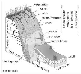
Fig. 5: The model of a normal fault with fault plane evolution indicators (modified from Giaccio et al. 2002).
