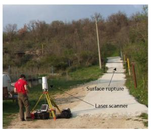
Fig. 1: Riegl LMS-z420i laser scanner set up at site PAG, one of the four surface rupture study sites.
