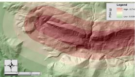
Fig. 6: Distribution of the generated PGA values based on the scenario of 1870 earthquake.
