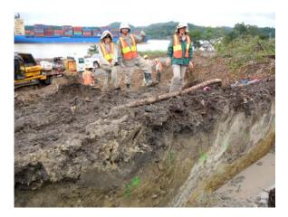
Fig. 6: Trench 48-B - the discovery trench, showing the fault (right) and the channel deposits (left), looking out over the Panama Canal in the background.
