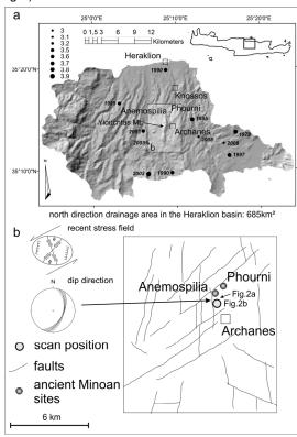
Fig. 1: Investigation area near Archanes in the Heraklion basin of Crete including earthquakes recorded since 1979 (a) (SRTM, USGS, www.usgs.gov) and the main faults, the LiDAR position, location and looking direction of photos (see Fig.2), dip direction of the scanned fault plane, recent stress field and ancient sites (b) (modified from Fassoulas, 2001; ten Veen & Meijer, 1998).
