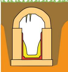
Fig. 2. Cross section of the roman aqueduct channel of Cologne, showing typical elements. The buried masonry channel is covered on the inside by a red layer of waterproof cement ("opus signinum"). Carbonate on the walls tapers upwards because of variable and gradually rising water level. In the Cologne case, the deposits indicate that the aqueduct ran for approximately 170 years (Fig. 3).
