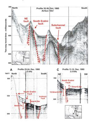
Fig. 5: Airgun 10 in<sup>3</sup> seismic profile (top) and 3.5 kHz profile (bottom) through the South Eratini Fault. Note that the 3.5 kHz profile shows vertical offset of the Holocene drape by about 5.5-4.5 m.
