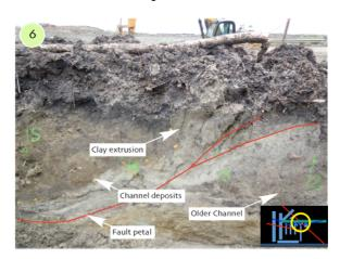
Fig. 7: Interpreted image of part of Trench 48-B showing the low-angle fault and the channel deposits on the hanging wall. The area shown as a "clay extrusion" is interpreted to be a weathered mole track from the MRE as it is intruded into, and deformed, the modern surface soils..
