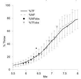
Fig. 1: Cumulative percentage of earthquakes that ruptured the surface for reverse (TF) and normal faulting (NF). Lines represent the model prediction, the symbols represent the data.
