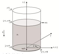
Fig. 1: Cylindrical tank
