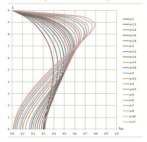
Fig. 6: Normalized flexible impulsive pressure Cif,h.
