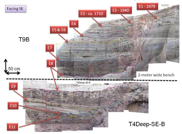
Fig. 3: Composite trench logs of T9B-SE (top) and T4Deep-SE (bottom) showing the remarkable Lake Cahuilla stratigraphy and the event horizons identified in these two exposures.
