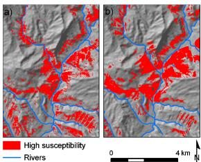
Fig. 5: Comparison of the results of the statistical and the data mining approach, a) InfoVal method, b) Bayesian networks. Both based on landslide data from 1962.
