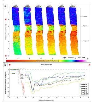
Fig. 2: Modelled postseismic deformation and rupture afterslip at PAG for the various time intervals. (From Wilkinson et al. 2010)
