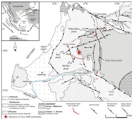
Fig. 1: Geological map of the study area showing lithology, active faults and surface ruptures during the Movri Mt earthquake.
