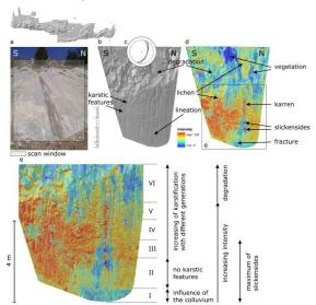
Fig. 3: Primary results of the LiDAR investigation based on the model in Fig.1. a) photo of the fault plane includes the LiDAR scan window, b) hillshade of the fault plane for geometrical and morphological analysis, c) dip direction of the plane, d) distribution of the backscattered signal with primary surface interpretation, e) primary interpretation of all fault plane conditions.
