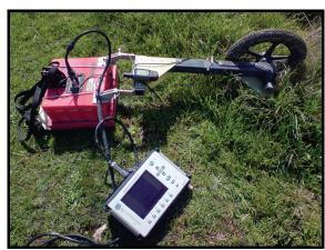
Fig. 3: GPR with 400 MHz antenna, survey wheel, SIR-3000 unit and GPS
