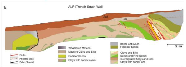
Fig. 2: South wall of trench ALF1, located at the Alfambras basin. Description of geology included in the figure.
