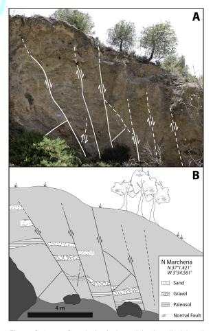
Fig. 4: Outcrop of an incised channel in the alluvial and colluvial fan in the north of Marchena. A: Photograph of the colluvial sediments and existing faults. B: Sketch of the same outcrop with a few traceable layers.
