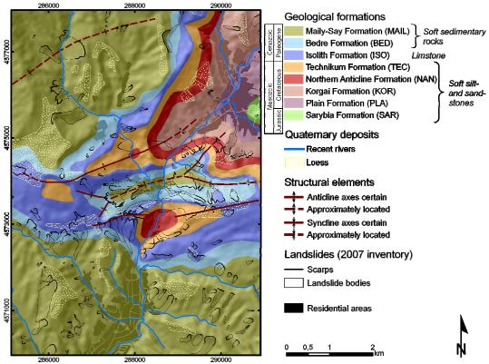
Fig. 4: Geological map of the working area showing distribution of loess deposits and outlines of landslides in 2007. Geology after de Marneffe (2010).
