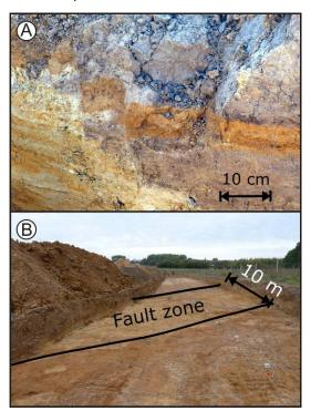
Fig. 5: A) Step-like offset clearly points to seismic deformation instead of soil creep. Displacement is about 5 cm. The offset reddish layer is made up of clayey-silty, loess material, 50 cm below the surface. B) The fault zone is clearly visible in the trenches, not only at the walls, but also on the floor. This enabled a very good correlation with the geophysical data and a precise analysis of subsurface features.
