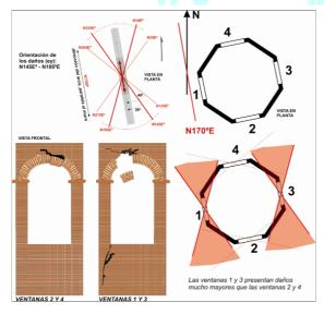
Fig. 5. Example of analysis of deformation structures and the results of the orientation assessment of the strain (San Juan's Church) (After Martínez-Díaz et al., 2011).
