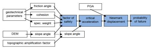
Fig. 1: Flow chart showing the steps involved in producing a seismic landslide hazard map; white: input parameters; blue: results (modified after Jibson et al., 2000).
