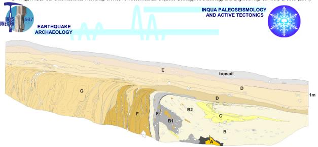
Fig. 3. Log of the trench F. See text for explanation of units A to E. Unit F – fault zone with tectonic breccia, G – metamorphic rocks
