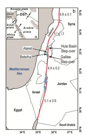
Fig. 1: a) Generalized tectonic framework of the Middle East. b) The DST (on land) from the Red Sea northward to the East Anatolian fault (EAF) in Turkey. Slip rate data are shown in black (Daeron et al., 2004, Ferry et al., 2007, Le Beon et al., 2010, Meghraoui et al., 2003).
