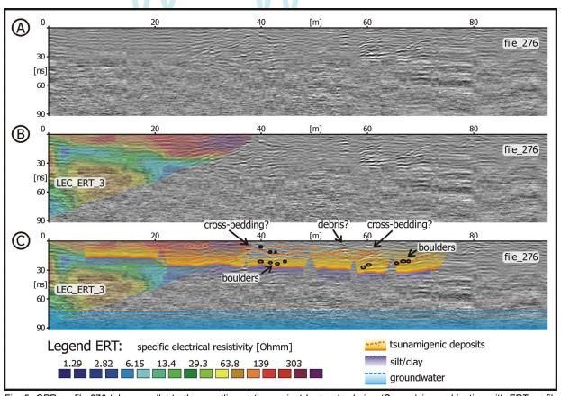
Fig. 5: GPR profile 276 taken parallel to the coastline at the ancient harbor Lechaion (Greece) in combination with ERT profile LEC\_ERT\_3: A) processed GPR data, B) processed GPR and ERT data; C) processed and combined analyzed data; yellow colored areas show tsunamigenic deposits; the base is illustrated by orange line; dashed orange lines refers to inner structures
