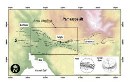
Fig. 2: The Delphi-Arahova-Amfissa Fault Zone. Fault plane projections for western and central-east part. After Valkaniotis (2009).
