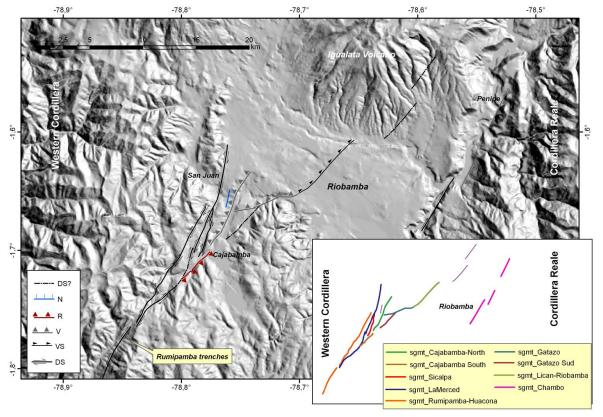
Figure 4: Sketch map of the northern extension of the PF within the Riobamba basin, and example of the morphological imprint of the fault. DS: segment with prevailing dextral component; N: with normal component (symbols on the downthrown block side); R: with reverse component; V: segment with undifferenciated vertical offset; VS: segment with vertical and dextral strike-slip component (symbols on the upthrown block side, for the 3 last).
