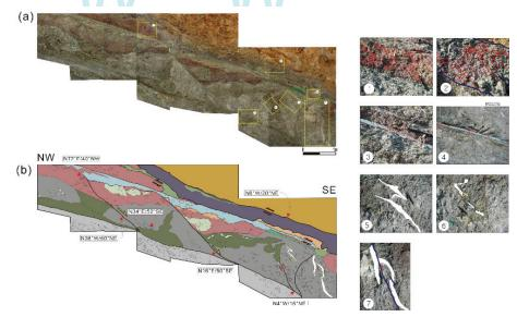
Fig. 3: Photomosaic (a), sketch (b) and sense indicators (c) of reactivated fault zone located at the new Weolseong nuclear power plant (Fig. 1).
