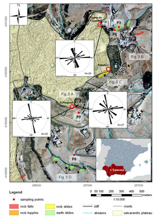
Fig. 2: Map of Carmona showing the sampling points for later geotechnical investigations, joint diagrams and the location of landslide phenomena illustrated in figure 3 (Gauss-Krüger coordinates).
