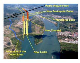
Fig. 1: Aerial view, looking NW, of the Pacific approach to the Panama Canal, showing the proposed location of the new locks, channel, and Borinquen Dam. The northerlytrending Pedro Miguel fault cuts through the proposed dam foundation about midway between the existing Miraflores and Pedro Miguel locks.
