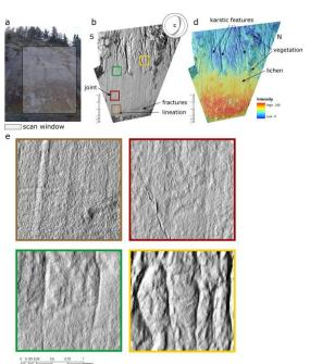
Fig. 4: a) photo of the fault plane includes the LiDAR scan window, b) hillshade of the fault plane for geometrical and morphological analysis, c) dip direction of the plane, d) distribution of backscattered signal with primary surface interpretation, e) brown, red, green and yellow boxes are demonstrate the different surface conditions on the fault plane in depending on the scarp height.
