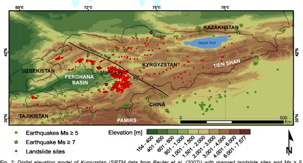
Fig. 2: Digital elevation model of Kyrgyzstan (SRTM data from Reuter et al. (2007)) with mapped landslide sites and  $Ms \ge 5$  earthquakes, based on data of the Kyrgyz and world seismic catalogue.
