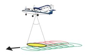
Fig. 1: Schematic diagram of LiDAR data acquisition
