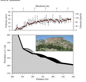
Fig. 2: (top) Red dots give median values of impact velocities of differently sized blocks at the location of the Roman mausoleum. (bottom) 2D model of the slope with trajectories of rocks of different size and form falling from the top of the cliff; a photo of which is shown in the insert.
