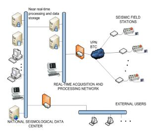
Fig.2. Real-time data transfer from seismic stations to NDC via Virtual Private Network (VPN) and three layer local network
