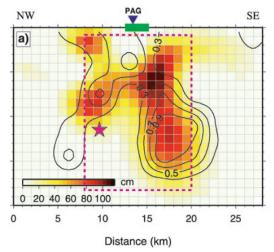
Fig. 5: Coseismic fault slip map derived from coseismic GPS data. The contours represent coseismic slip (m). Note the location of study site PAG at the surface and the coseismic slip deficit (white patch) within the fault zone beneath it. (Figure adapted from Cheloni et al, 2010)
