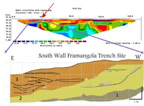
Fig.4. Geoelectric tomography profile (using Schlumberger method) at Framangola site at the alluvial plain, strongest contrast coincides with previously identified fault trace; the trench units identified also correlate with the tomography (1) Clays and fine silts; (2) Very coarse Gravel (3) Silty sandy & fine conglomerate
