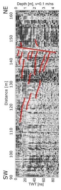
Fig. 3: 270 MHz GPR profile (64) crossing the fault with an angle of 45°.
