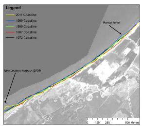
Fig. 5: Synthetic image with all the traced coastlines at a part of the study area where Pineios river used to flow into the sea before 1800's.
