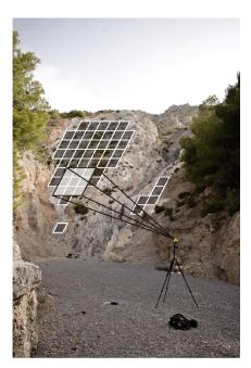
Fig. 3: Illustration of a laser distance measurement. Exhumed scarp near the natural monument "Nigüelas Fault"
