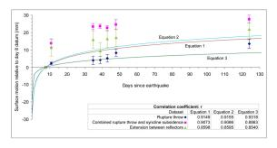
Fig. 4: Surface motion measurements of rupture throw (purple diamonds), hangingwall syncline subsidence (pink squares) and extension between reflective targets (green triangles), derived from the modelled data in Fig 2. Our measurements are compared to data for the three theoretical and empirical models for afterslip shown in figure 3. (Figure from Wilkinson et al. 2010)
