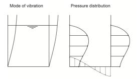
Fig. 4: Flexible impulsive pressure - Mode of vibration and pressure distribution.
