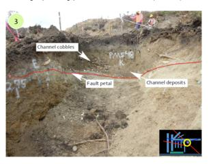
Fig. 9: Interpreted image of the end of Trench 48-K, with 48-B (Fig. 7) ~ 1 meter on the other side (to the south) of the trench. This image shows the channel deposits still above the fault trace.
