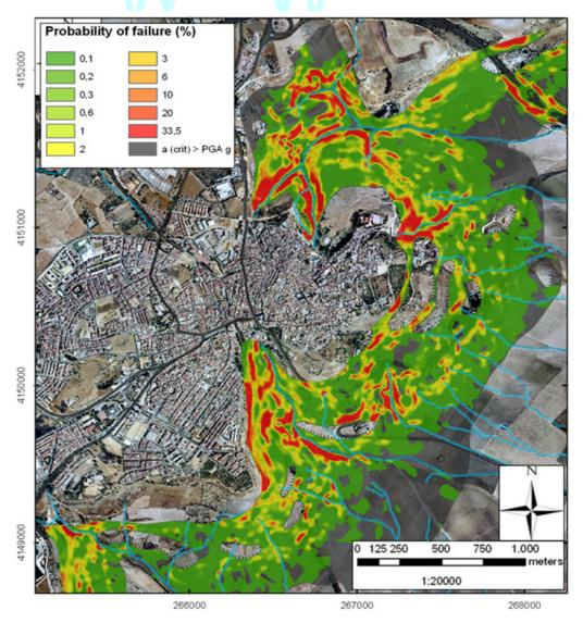
Fig. 4: Probabilistic landslide hazard map showing the probability of failure in case of an intensity-IX (EMS) earthquake under fully water saturated conditions (Gauss-Krüger coordinates).
