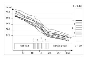
Fig. 5: Twelve perpendicular profiles from the 120 m long Delphi scarp segment show the horizontal and vertical discontinuity of the fault plane. 1) Variations of the free face fault plane. 2) Top knick point of the free face to the foot wall. 3) Bottom knick point of the free face to the hanging wall.
