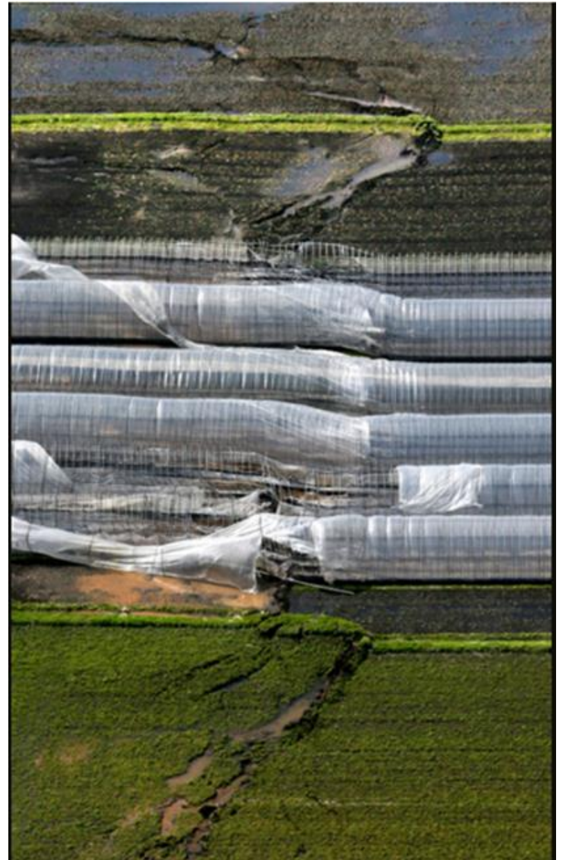
Surface faulting during 2016 Kumamoto Earthquake - Compilation by S. Baize (IRSN)
