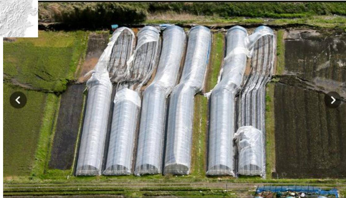
Surface faulting during 2016 Kumamoto Earthquake - Compilation by S. Baize (IRSN)
