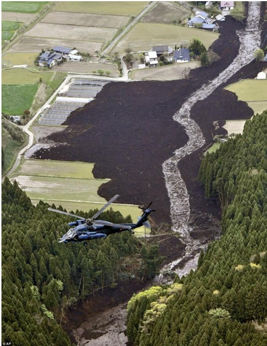
A flowslide triggered by the Kumamoto earthquake, via AP
