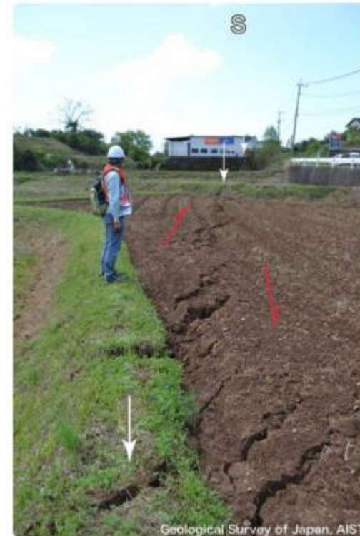
13-Right-lateral displacement seen in the rice paddies of the photo 13 Takagi village. Picture taken toward the south direction. Right-lateral displacement amount is about 50 cm. (2016 April 17 shooting)
