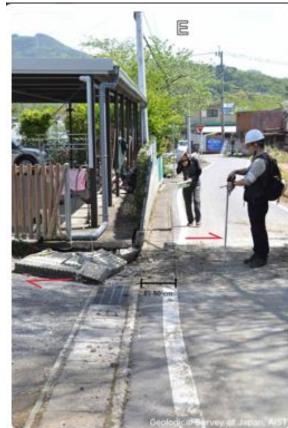
14- Right-lateral displacement seen in the pavement of Kamikoya village. Picture taken toward the east direction. Right-lateral displacement amount of time on the basis of the gutter is about 50 cm. (2016 April 17 shooting)
