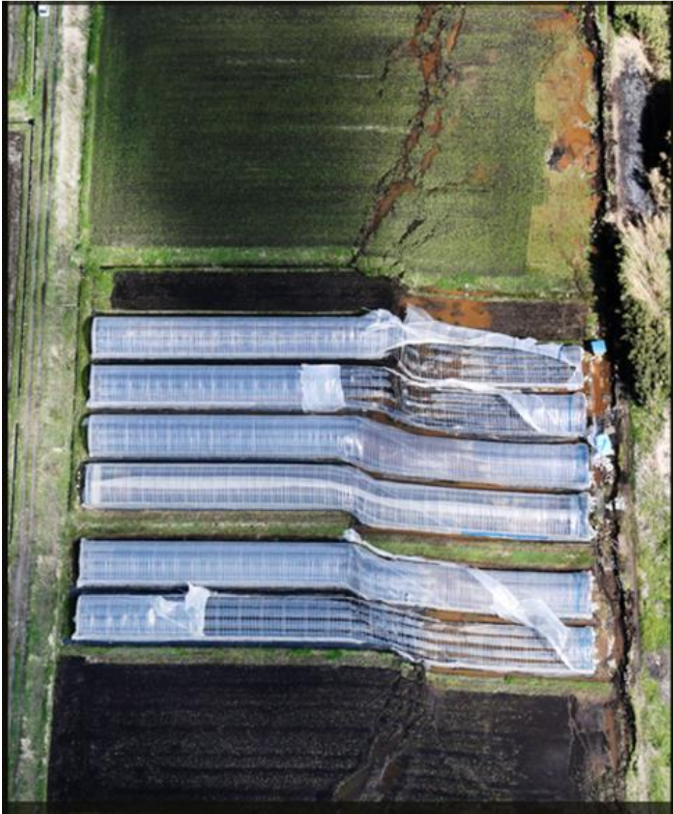
Surface faulting during 2016 Kumamoto Earthquake - Compilation by S. Baize (IRSN)
