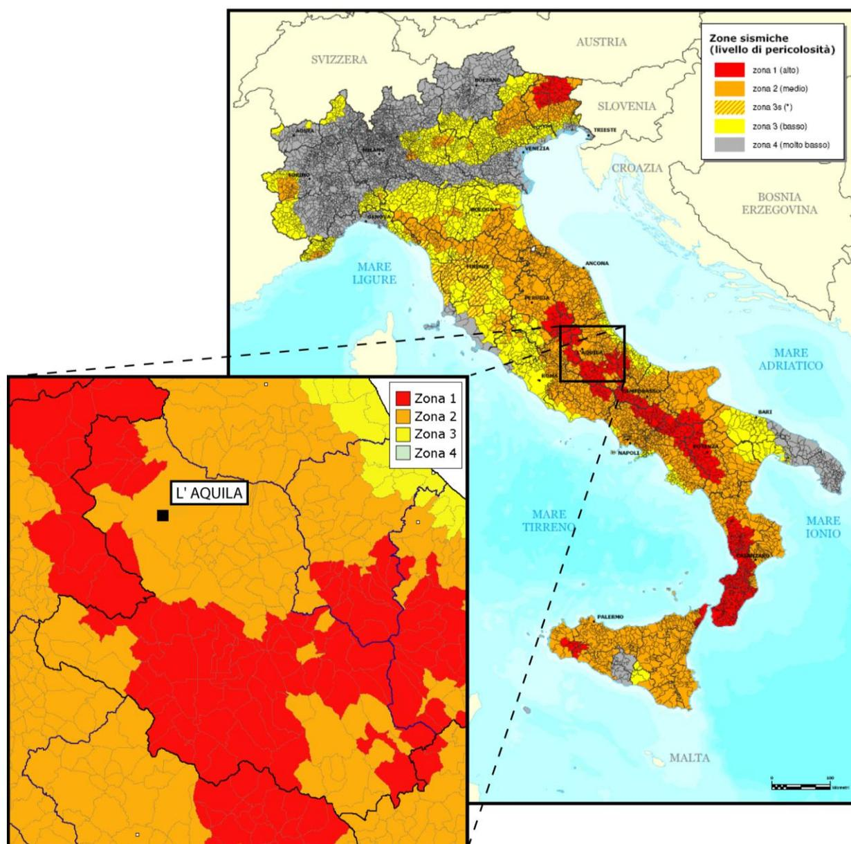
Figure 3. Seismic hazard map of the Italian territory (Protezione Civile Nazionale, 2006). The area of L' Aquila belongs to seismic zone 2 and requires a design level value of 0.25g of peak horizontal ground acceleration.
