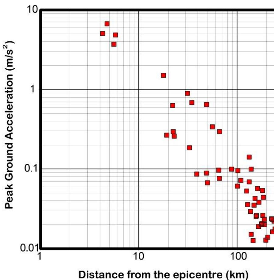
Figure 18. Diagram showing the PGA values versus distance in the epicentral area.
