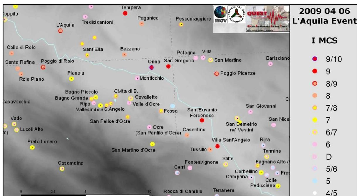
**Figure 12.** View of the macroseismic intensities expressed in MCS (Mercalli-Cancani-Sieberg) values (Quest 2009).
