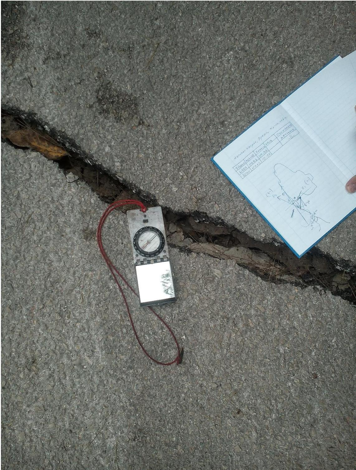
**Figure A10** Field photo of 7cm wide tensional crack at Dragano village. Extension azimuth is N130°E. Nadir view. Date photo was taken 22 Nov. 2015.
