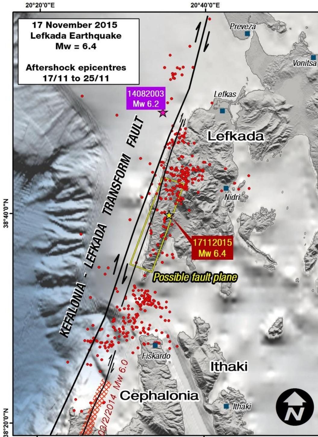
Figure 1. The 17th November 2015 Lefkada main earthquake (yellow star) and aftershock revised epicentres recorded by National Observatory of Athens (NOA). Dextral faults along the Cephalonia-Lefkada Transform boundary are shown as black lines.
