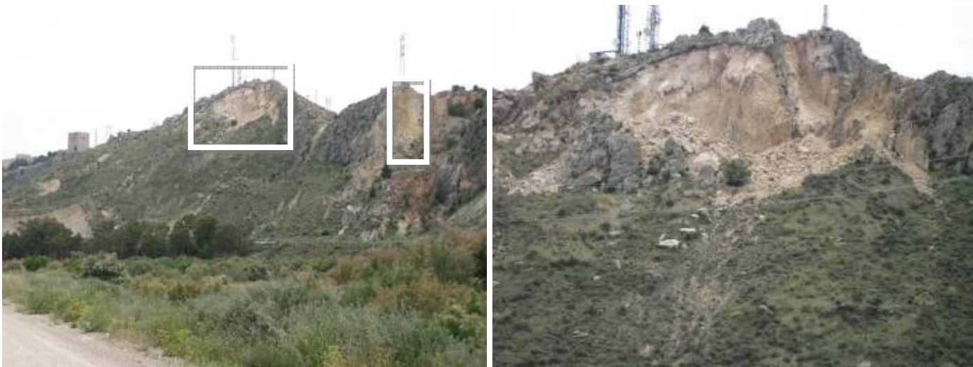
Figure 4.4.1a: Rock-falls and debris on the summit of the north slopes of the Pantano de Puentes road. Their attribution to the earthquake is presumed. The westernmost one (on the right on the first photo) corresponds in part with a previous instability.
