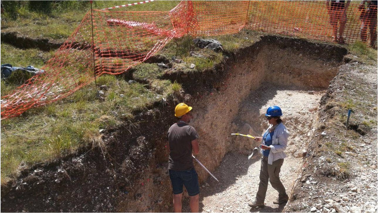
Fig.5: Francesca Cinti (INGV) shows the surface faulting occurred along a secondary fault during the 2016 October 30 th earthquake, on the trench wall at Pian Perduto site (MC) in the morning of 21 st of July, 2017.
